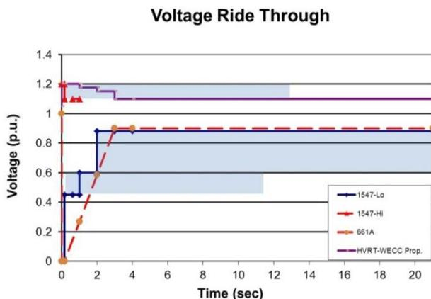
**Figure 9. Graphical representation of voltage ride-through as defined in IEEE 1547 [12]**
