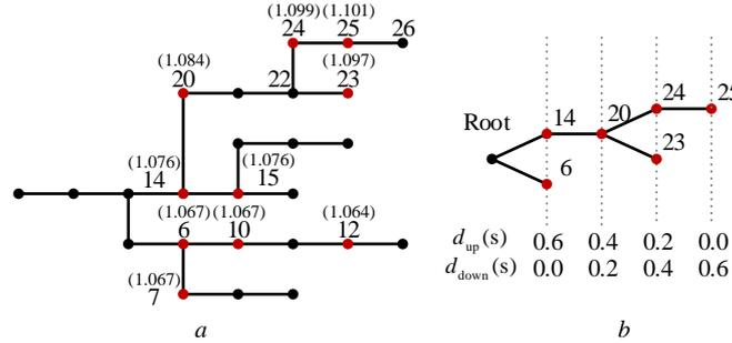
Figure 4: Time delay allocation. a) Network topology with voltages and b) the corresponding tree with the calculated time delays.
