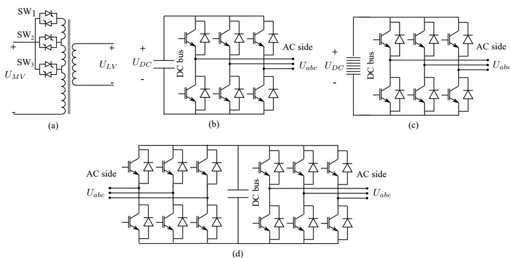
**Figure 4.** Power electronic devices incorporated in the smart grid distribution system: (a) solid state tap changer (SSTC); (b) three-phase, three-wire STATCOM; (c) three-phase, three-wire BESS; and (d) DC link composed of two back-to-back VSCs.
