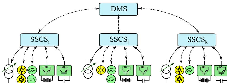
Figure 5. Hierarchical control of active distribution systems.
