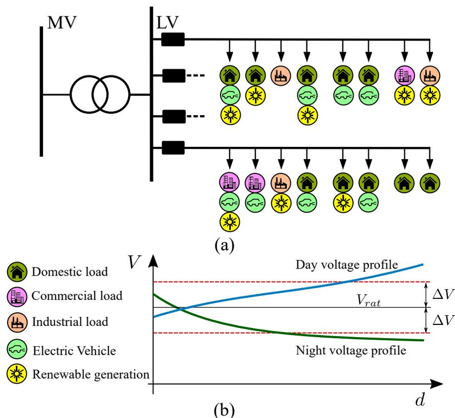
**Figure 2.** Two-way LV distribution feeders: (a) one-line diagram; and (b) voltage profile along the feeder.
