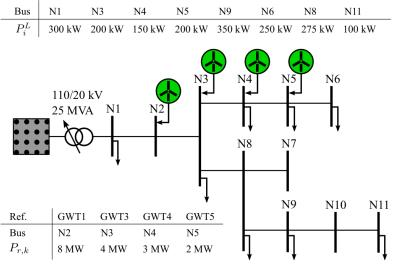
Power injection is limited by the maximum current admissible at the header
