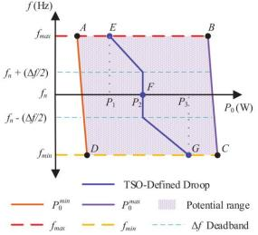
CCC EASY-RES // The EASY-RES approach for aggregation and disaggregation of Inertia and PFR
