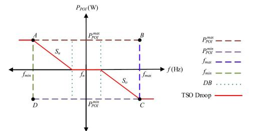
$$\Delta P(t) = \begin{cases} S_u(\Delta f + DB)G_u(t), & \text{if } f \leq f_n - DB \\ 0, & \text{if } f_n - DB < f < f_n + DB \\ S_o(\Delta f - DB)G_o(t), & \text{if } f \geq f_n + DB \end{cases}$$
